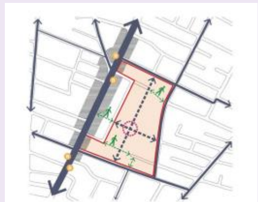
Well-designed places have a hierarchy of well-connected routes, such as boulevards, streets, roads, avenues, mews and courts. New developments help to reinforce or extend the movement network. For pedestrians and cyclists, direct links create good connections to public transport and promote active travel, particularly where they are along routes with low levels of vehicular traffic.
